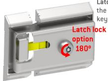
Latch retention option. This system allows the latch to be left in the open position, after turning the key 180° to the right. This allows the padlock to be left open.
